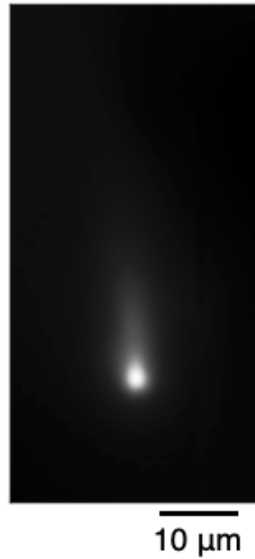
Figure ED3: SQUID point spread function. Image of the SQUID point spread function, K_{PSF} extracted from imaging a superconducting vortex. The SQUID pickup loop has an inner diameter of 1.5 \mu\text{m} , giving micrometer scale spatial resolution for magnetic imaging.
