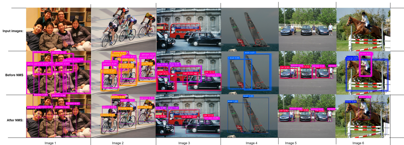
Fig. 5: Sample MultiGridDet output on randomly selected Pascal VOC 2007 test set images. As seen from the figure the first row shows six input images, whereas the second row shows the prediction of the network before non-max-suppression (NMS) and the last row shows the final bounding box prediction of MultiGridDet on the input image after NMS thresholding.
