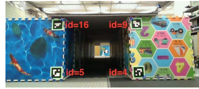
Fig. 3. The detected ArUco markers at the tunnel entrance and the corresponding marker IDs.
