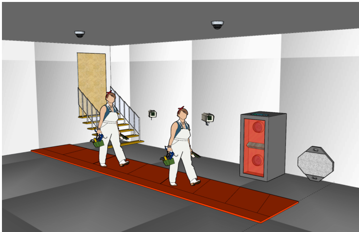
Fig. 5. Example of gait data acquisition environment. The scene comprises the following devices: sidewall cameras, followed by a multi-spectrum photographic sensor. The roof accommodates velocity sensors and gyroscopes, which measure the space-time relationship during the walk. Finally, the floor is equipped with a carpet-like sensor for collecting the foot pressure on the ground, completing the gait cycle.
