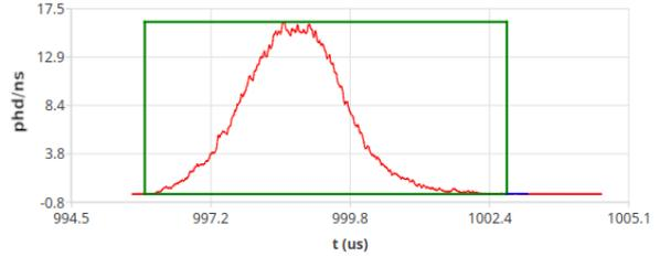
(b) Typical shape of a low-energy S2 pulse.
