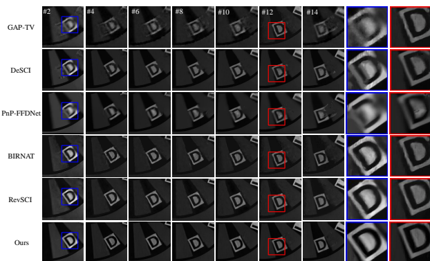
Figure 6. Comparison of selected reconstruction video frames of real data Wheel with the spatial size of 256 \times 256 \times 14 .
