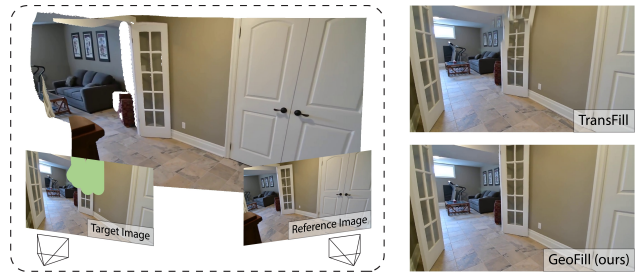
Figure 1: Given a reference image and a target image with hole, GeoFill utilizes predicted correspondence matching and depth maps to estimate a 3D mesh and relative camera pose and intrinsics. Compared to TransFill, the previous state-of-the-art approach, GeoFill handles complex scenes better by iteratively refining predicted depth maps and relative pose.
