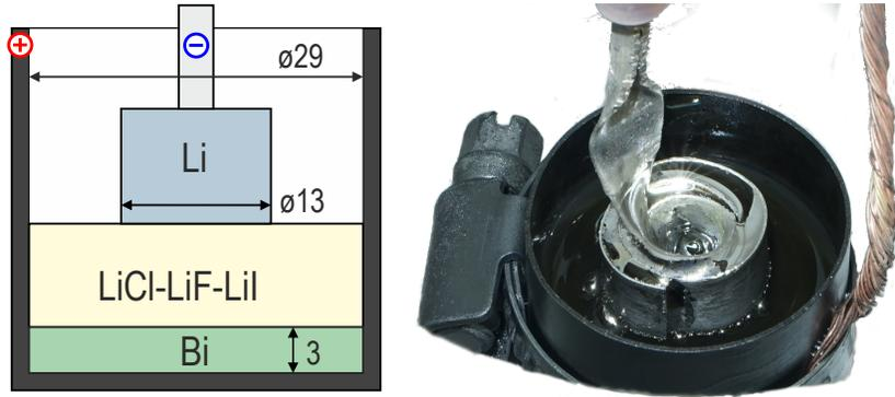
Figure 9: Setup and dimensions (in mm) of the small Li-Bi laboratory cell (not to scale). The thicknesses of positive electrode and electrolyte are given for the start of the charge phase (figure 10).
