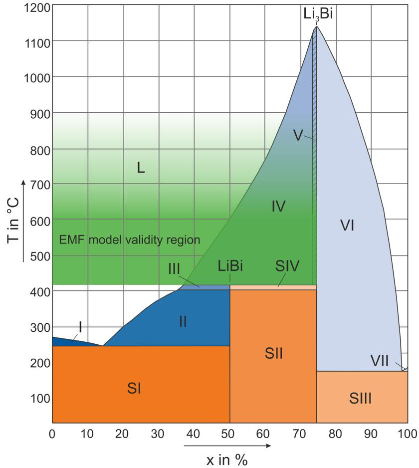
Figure 2: Phase diagram of Li-Bi according to [42] with different cell voltage areas and the region of validity shaded in green. L denotes the liquid phase.
