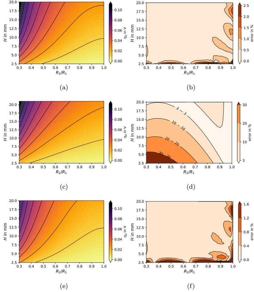
Figure 5: Fitted ohmic overpotential for a cylindrical cell (a) and corresponding error (b), analytically computed ohmic loss for the same cell (c) with error (d) and fitted ohmic overpotential for a square cell (e) with error (f). In the examples (a, c, e),  $\sigma = 1 \text{ S/cm}$ ,  $I = 1 \text{ A}$ ,  $R_1 = 5 \text{ cm}$  and  $L_1 = 10 \text{ cm}$ .
