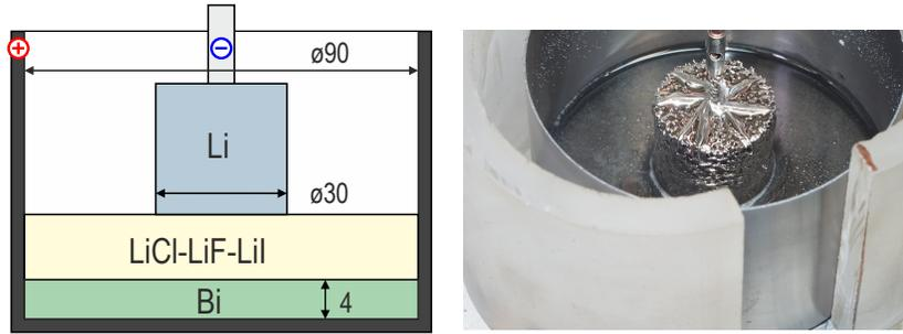
Figure 11: Setup and dimensions (in mm) of the large Li-Bi cell (not to scale). The layer thicknesses are given for the start of discharge in figure 12.
