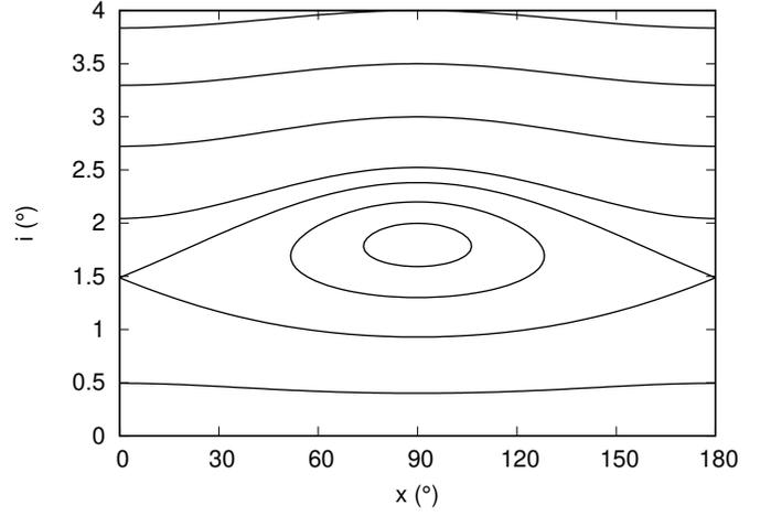
Fig. 3: Level curves of the Hamiltonian (24) for Phobos (Table 1), for a semi-major axis  $a = 2.61686R$ , and assuming an obliquity  $\varepsilon = 90^\circ$  for Mars.
