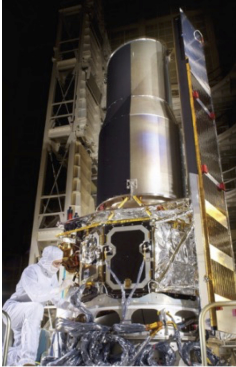
Fig 3 The assembled Spitzer observatory being prepared for thermal vacuum testing at Lockheed Martin in Sunnyvale, CA. The photograph illustrates the key features of the thermal control system up to and including the outer shell of the telescope. These include the chevron-shaped solar panel, the solar panel shield immediately behind it, and the telescope outer shell, with its anti-solar side painted black to maximize its infrared emissivity. Also visible between the spacecraft and the outershell is the spacecraft shield which isolated the outer shell from the spacecraft. Credit: NASA.
