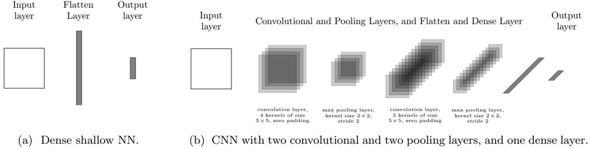
FIGURE 3. Architectures of the NNs used in the experiments of Section 4.3, cf. [15, Section 4].
