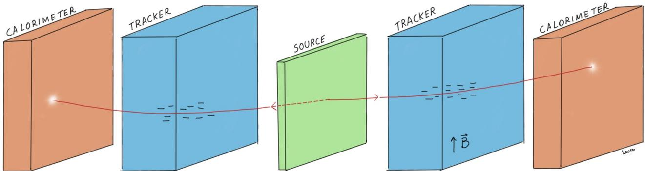
FIG. 26 Artistic illustration of a tracking-calorimeter detector and its  $0\nu\beta\beta$ -decay detection concept. The charge, momentum, and energy of the particles ejected by the source is measured through a combination of magnetic-field trackers and calorimeters. Image courtesy of Laura Manenti.
