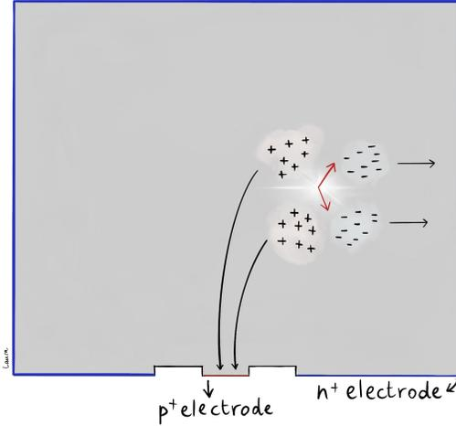
FIG. 22 Artistic illustration of a high-purity Ge (HPGe) detector and its  $0\nu\beta\beta$ -decay detection concept. Electron and hole clusters created by ionization are collected to the electrodes by an electric field. Image courtesy of Laura Manenti.
