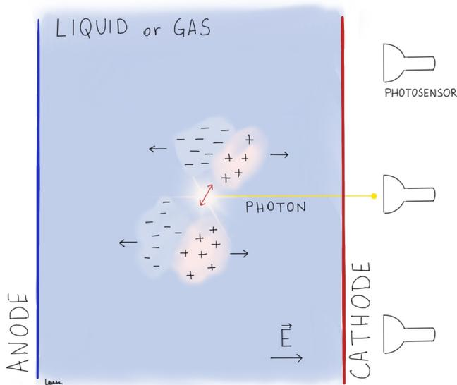
FIG. 23 Artistic illustration of a Xe time projection chamber and its  $0\nu\beta\beta$ -decay detection concept. Electron and hole clusters created by ionization are collected to the electrodes by an electric field. In addition, scintillation light is detected by light sensors, providing the timing of the event. Image courtesy of Laura Manenti.
