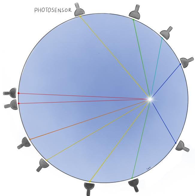
FIG. 24 Artistic illustration of a large liquid scintillator detector and its  $0\nu\beta\beta$ -decay detection concept. The position of an event can be reconstructed through the time of flight of the scintillation photons. Image courtesy of Laura Manenti.
