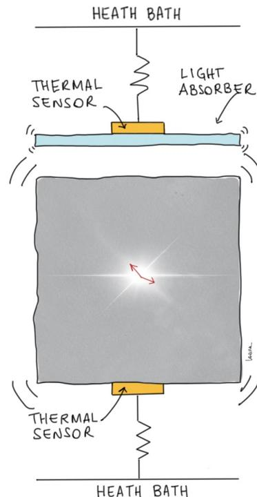
FIG. 25 Artistic illustration of a cryogenic calorimeter and its  $0\nu\beta\beta$ -decay detection concept. Phonon and scintillation light signals are read-out through superconductive thermal sensors. Image courtesy of Laura Manenti.
