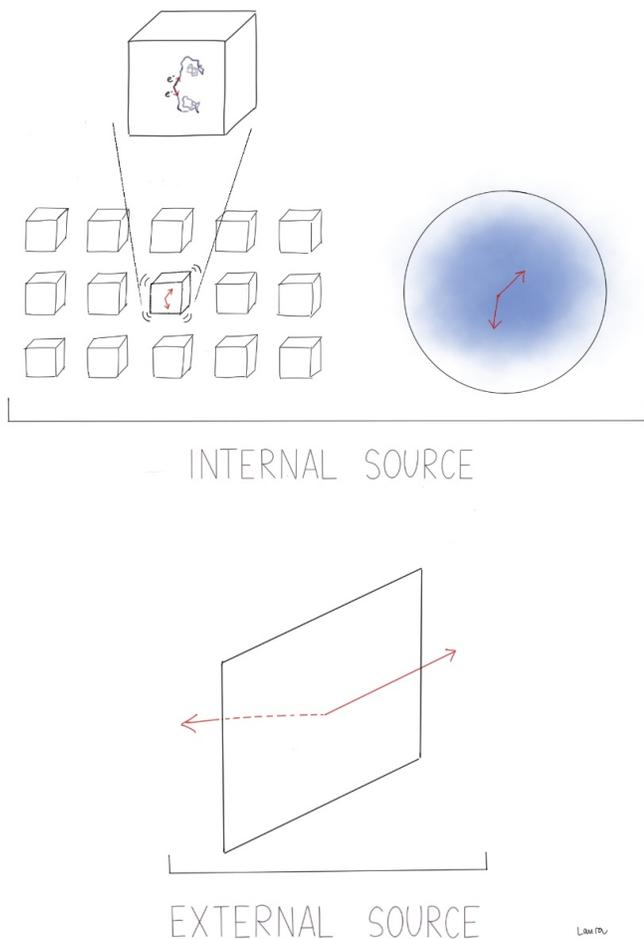
FIG. 13 Artistic rendition of the three detector concepts used to search for  $0\nu\beta\beta$  decay: internal-source experiments using solid state detectors (left) or monolithic liquid or gas detectors (center), and composite experiments (right) for which the source is external to the detection apparatus. Image courtesy of Laura Manenti.
