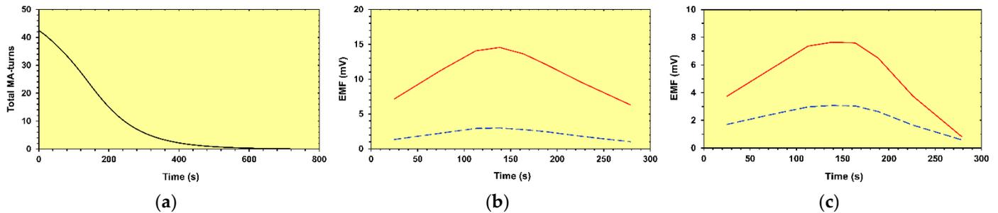
**Figure 4.** Modelled (a) CMS coil current fast discharge; (b) minimum (dashed) and maximum (solid) EMF voltages per one-turn flux loop on the blocks of the CMS barrel wheels; (c) minimum (dashed) and maximum (solid) voltages per one-turn flux loop on the  $18^\circ$  segments of the CMS endcap disks [12].
