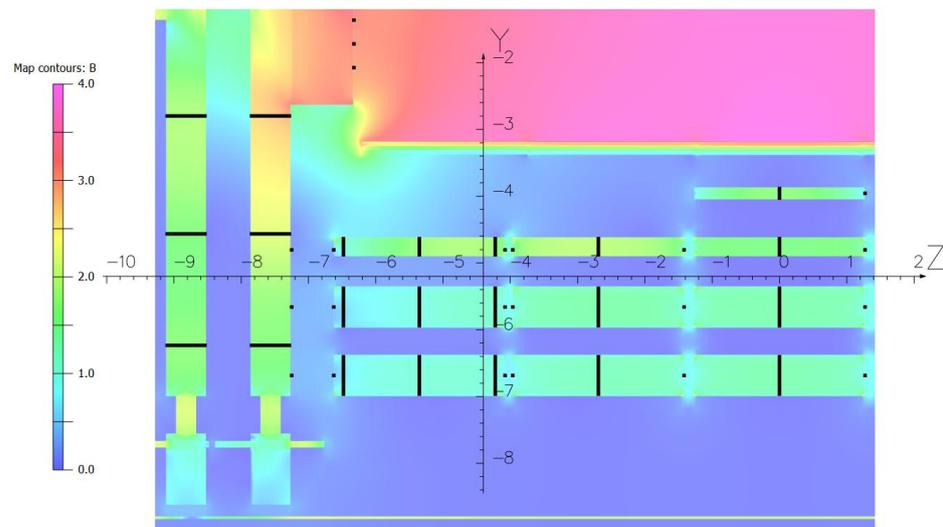
**Figure 10.** The magnetic flux density distribution in the longitudinal sections of the CMS detector. The colour scale is from zero to 4 T with a unit of 0.5 T. The black lines display twenty-two flux loop cross sections. The black squares denote the projections of the 3D Hall probe positions to the vertical YZ-plane. The values along the vertical Y-axis and horizontal Z-axis are presented in meters and are counted from the centre of the superconducting solenoid.
