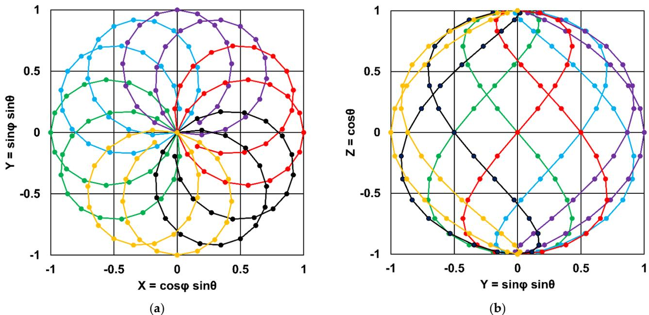
**Figure 3.** Trajectories of the magnetic flux density unit vector in the calibrator head local coordinate system: (a) in the XY-plane; (b) in the YZ-plane. Different colors correspond to six complete turns of the calibrator head with the outer axes. Markers denote the increments of  $9.375^\circ$  in azimuth  $\varphi$  and  $11.25^\circ$  in polar  $\theta$  angles used to prepare the plot.
