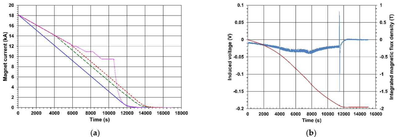
**Figure 13.** (a) CMS magnet current discharges from 18.164 to 0 kA made on July 17 and 18, 2015 (blue smooth line), September 21 and 22, 2015 (green dashed line), September 10, 2016 (red short-dashed line), and November 30, 2017 (magenta dotted line) [30]; (b) Induced voltage (left scale, noisy curve) and the integrated average magnetic flux density (right scale, smooth curve) in the cross section at  $Z = -2.691$  m of the first layer block of the W-1 barrel wheel [30].
