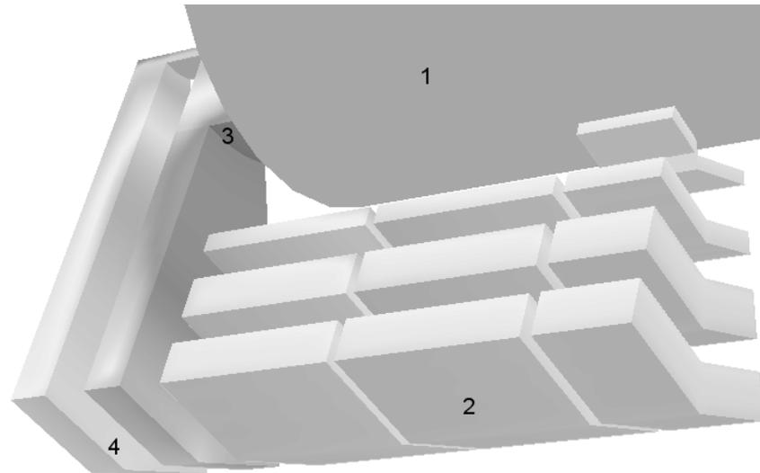
**Figure 6.** ELEKTRA model used for the yoke eddy current calculation [29]. CMS coil (1), the yoke sectors of the barrel wheels (2), nose disk (3), and two endcap disks (4) are presented in the model.
