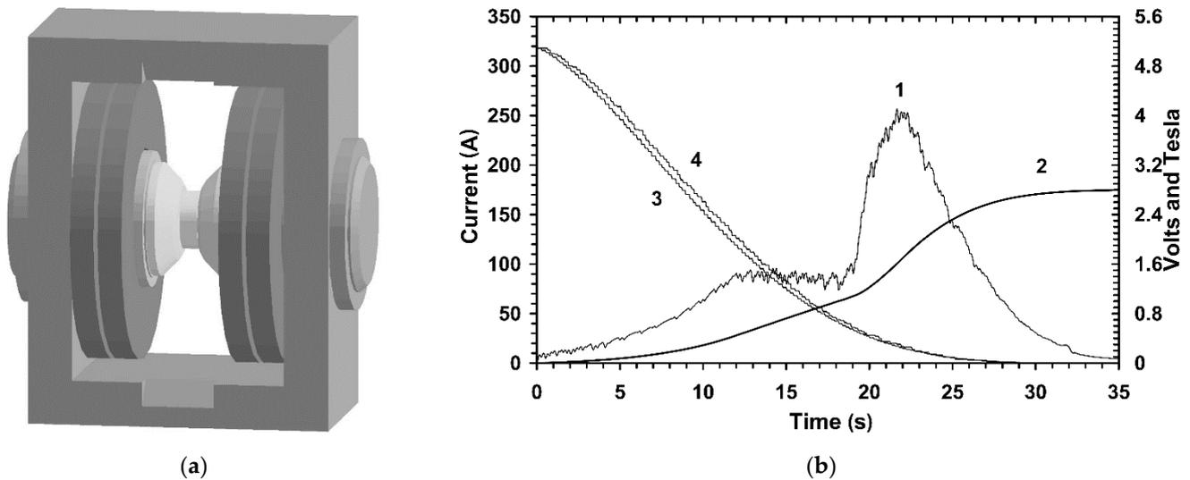
**Figure 5.** (a) 3D model for the test magnet with the steel sample disk inserted between the pole tips [12]; (b) Induced voltage (curve 1) and the integrated magnetic flux density (curve 2) when the test magnet current ramped down from 320 A to zero during 32 s. Curve 3 shows the requested current from the control software. Curve 4 corresponds to the measured current read-back [12].
