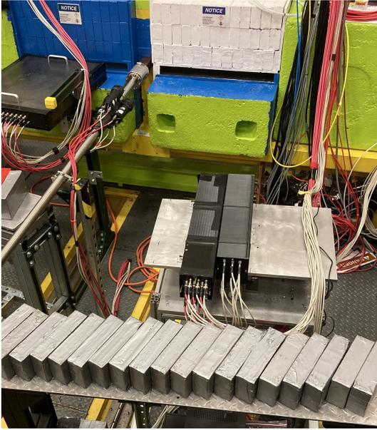
**Fig. 2** The  $\text{PbWO}_4$  EIC EM calorimeter prototype (on the left) installed in the Hall-D downstream of the Pair Spectrometer (PS).
