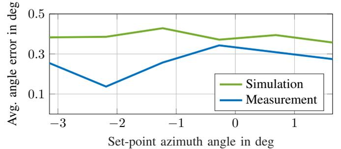
(a) Simulated and measured azimuth angle error.
