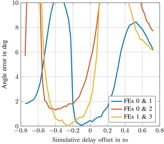
Fig. 3. Measured angle error over artificial delay offset used for phase coherency calibration of the respective RTS front ends.
