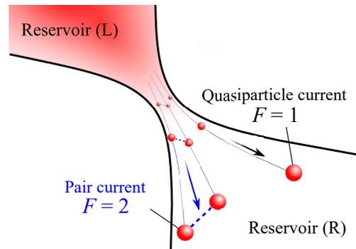
FIG. 1. Strongly interacting quantum gases (reservoirs L and R) with a large chemical-potential bias in between. The Fano factor  $F$  can be regarded as an indicator of the current carrier, i.e., quasiparticle current ( $F = 1$ ) and the pair current ( $F = 2$ ).
