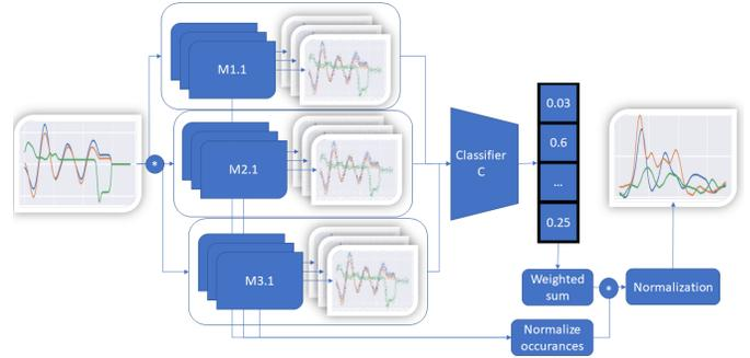
Fig. 1. **TimeREISE**. A set of masks with different density and granularity is applied to the input using an exchangeable perturbation function. The default perturbation is an elementwise multiplication. The masked input is passed to a classifier and the classification score is retrieved. The classification score is multiplied with the masks and normalized by the number of feature occurrences. Finally, the attribution is normalized to scores between zero and one.
