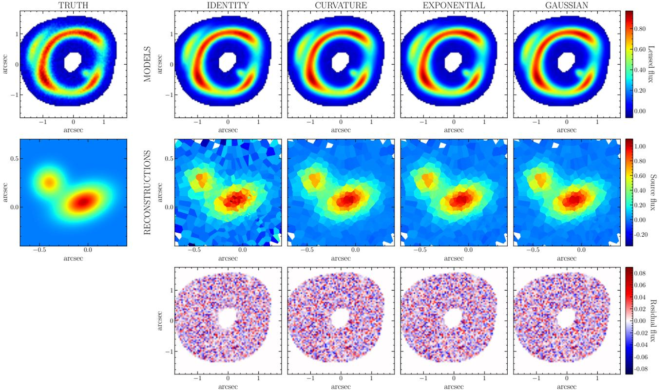
**Figure 1.** Lensed images (top), source (middle), and residuals (bottom) for the mock data (truth) and the reconstructions with different source regularization kernels: identity, curvature, exponential, and Gaussian. The source brightness, shown as Voronoi cells of an adaptive grid (see Section 2.1), has been reconstructed using  $n = 3$ . The corresponding parameters for the lens potential and the source regularization are shown in Table 1.
