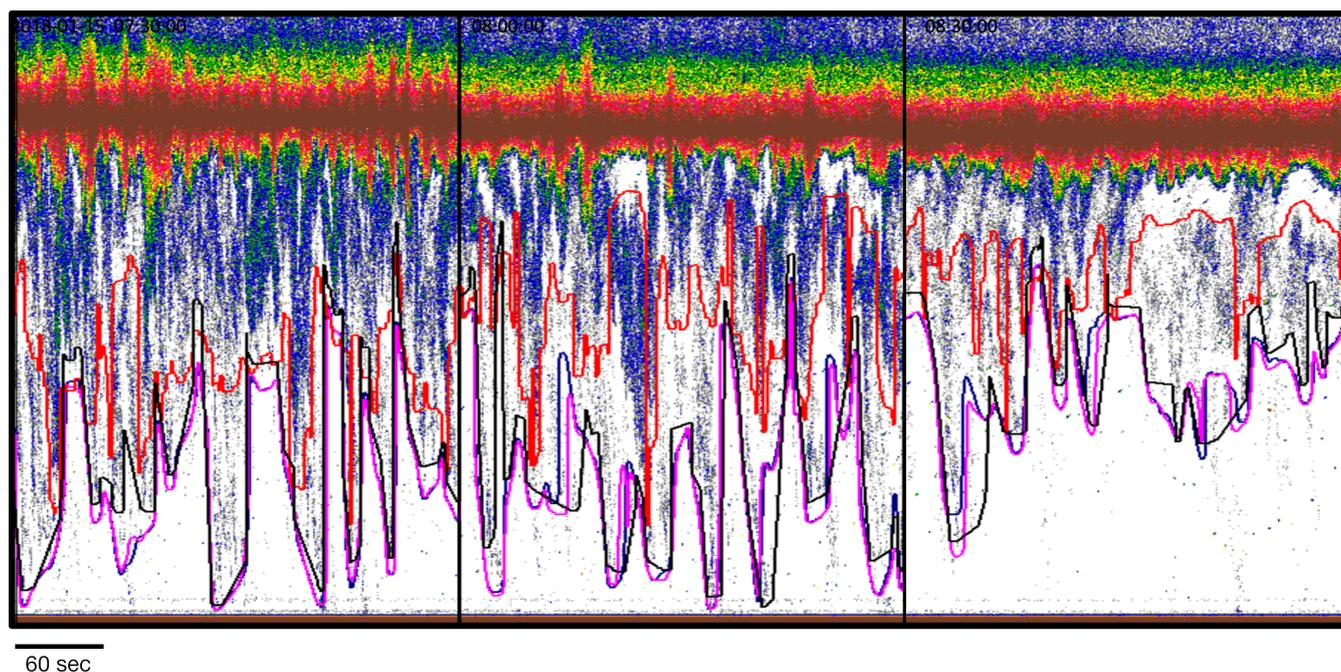
**Figure 5** Echogram demonstrating that the entrained-air line as calculated by the two Echofilter models (Upfacing@400ep: pink; Bifacing@700ep: blue) is a pronounced improvement over that produced by Echoview (red line), and much closer to the target line created by the analyst (black). Data: stationary data with echosounder in upfacing orientation, recorded for 5 minutes every half hour at the Minas Passage site.
