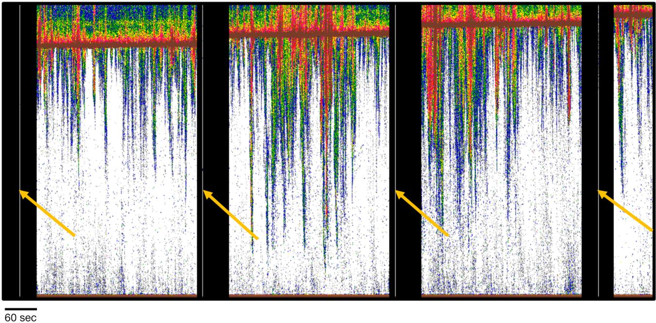
**Figure 7** Passive data regions (black vertical bars) as identified by Echoview algorithms. Note the white vertical lines marked by yellow arrows within the black passive data regions. The white vertical lines are single pings or a few pings misclassified by the Echoview algorithm. Data: stationary data with echosounder in upfacing orientation, active data recorded for 5 minutes and passive data for one minute every half hour at the Minas Passage site.
