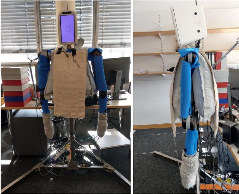
Fig. 3. Front and side views of HuggieBot 2.0 [13] without the robe and sweatshirt so that the HuggieChest, heating pads, and foam arm padding can be clearly seen.
