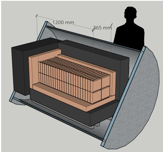
**Fig. 6.** Sketch of a pressure vessel holding the full detector load and an inner lead and copper shields. The dimension lines refer to the “stacks” of supermodules, which in this sketch cover 120×36.5 cm. An external shield of ~60 cm of HDPE (or equivalent absorption power of water) and an additional ~10 cm of lead is not shown.
