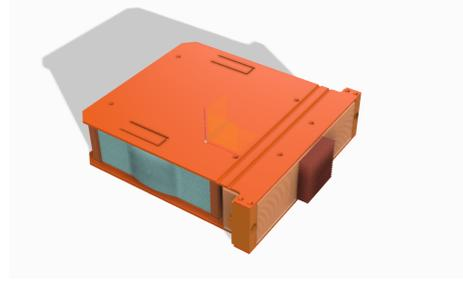
**Fig. 5.** (left) Design of the Oscura Multi Chip Module (MCM) with 16 sensors mounted on a 150 mm silicon wafer. (right) Oscura Super Module (SM) with 16 MCMs supported and shielded with electroformed copper.
