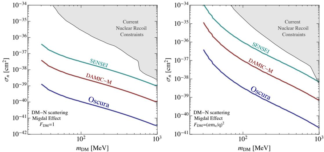
**Fig. 4.** Projected sensitivity to dark-matter-nucleus scattering of Oscura, assuming a 30 kg-year exposure (blue). We assume a two-electron threshold and zero background events. Projected sensitivities for SENSEI (DAMIC-M) are shown in cyan (red). The projections have been scaled from [47]. Existing constraints are shaded gray [6, 27, 33, 48–50]. The left (right) plot assumes the DM-nucleus interaction is mediated by a heavy (light) mediator.
