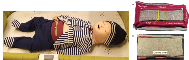
Fig. 1. (left) A smart-fabric Bellyband and (right) Bellypatch can be integrated into wearable garments to enable wireless and passive biomedical monitoring in infants.
