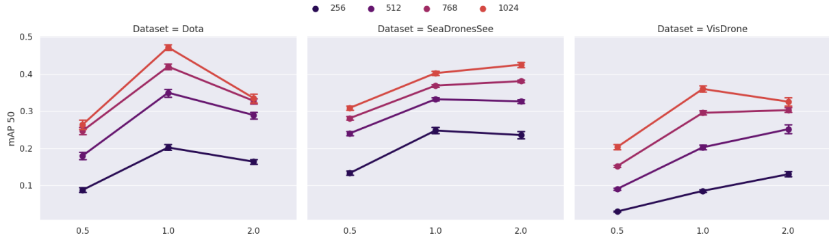
Figure 13: Image Size: Faster R-CNN trained with different training image sizes and validated on validation image size = x \times training image size. The y-axis shows the mean Average Precision (mAP).
