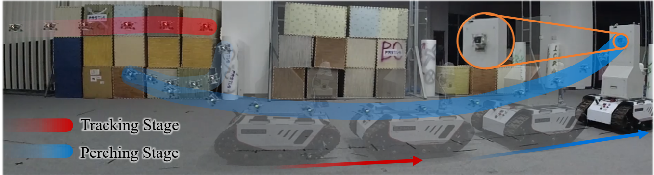
Fig. 1: Aerial perching on the vertical surface of a moving platform. The drone first tracks the ground vehicle (red) and then plans and carries out the perching trajectory (blue) when triggered. Since our drone has low thrust-to-weight ratio (1.7) and is close to the ground, our planner generates a swing-shaped trajectory guaranteeing both safety and dynamic feasibility.
