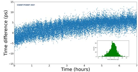
Fig. 7. Variation of the time difference between the arrival of clock pulses at Rx1 and Rx2 over 7 h. The maximum time difference is 5 ps due to fiber length variations. Inset: histogram of the time difference over a 900 s time scale indicates a timing jitter of 2 ps.
