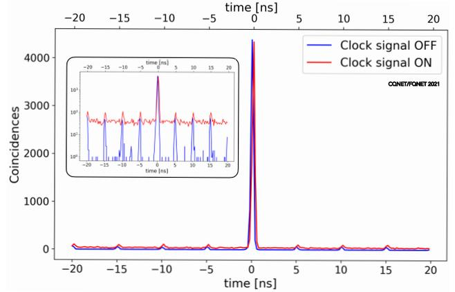
Fig. 6. Coincidence histogram with the clock distribution enabled and disabled. The small time delay between the two histograms is due to a small difference in trigger voltage threshold. Inset: Coincidence histogram with a log vertical scale reveals the Raman noise from the clock pulses.
