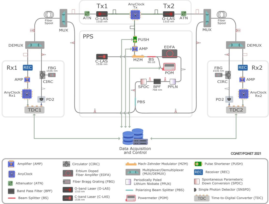
Fig. 2. Schematic of fiber-based three-node quantum network and synchronization system. See main text for description. Clock pulses are indicated by top hats while grey and red Gaussian-shaped pulses indicate single photons and second-harmonic (768 nm) light, respectively.
