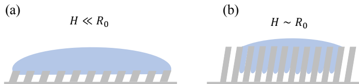
Figure 9: Schematic description of the wetting and rebound scenario on microstructures (a) with small height compared to the radius of the droplet (b) with comparable height to the radius of the droplet.
