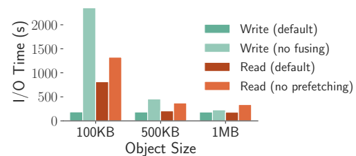
Figure 9: Effect of I/O optimizations in Ray.
