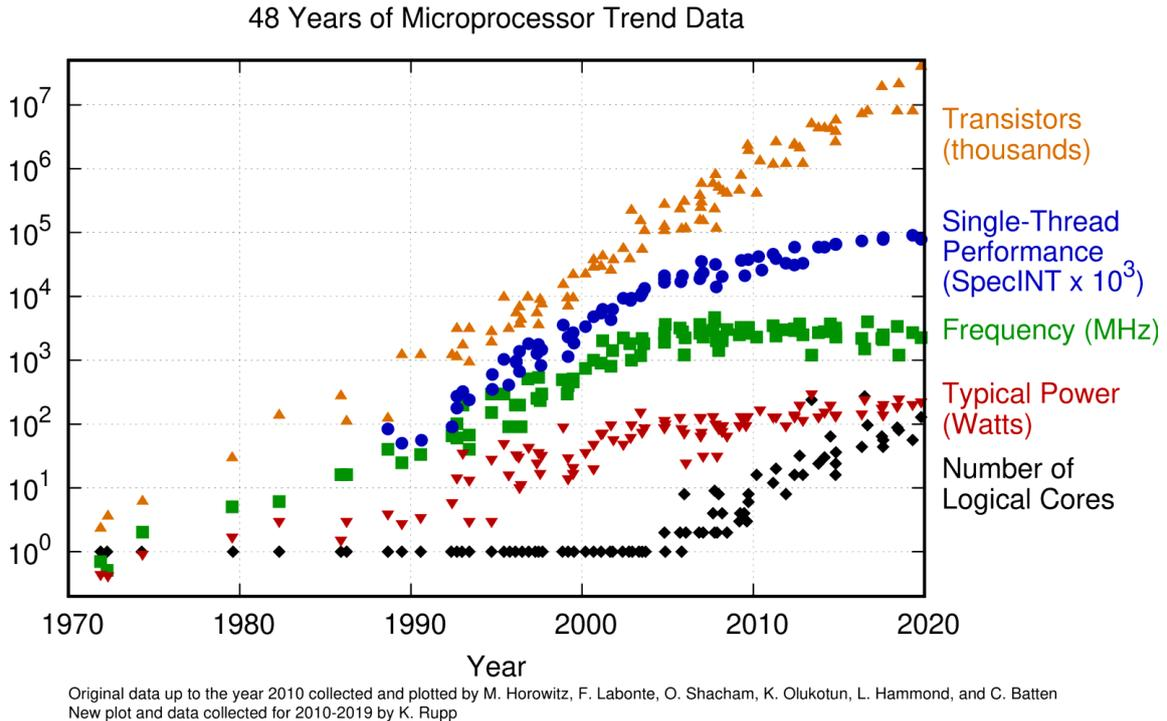
**Figure 1.** Microprocessors reach the power wall limit circa 2010
