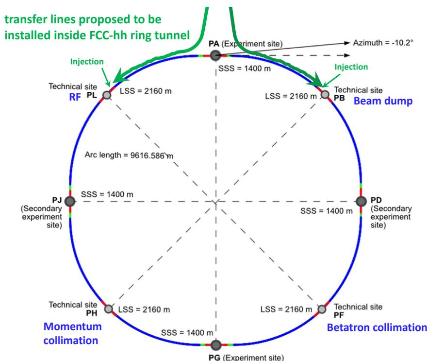
Figure 4: Sketch of the proposed eight-point FCC-hh layout.
