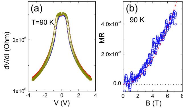
FIG. 3. (a) Differential current-voltage characteristics,  $dV/dI(V)$ , at  $T = 90$  K in magnetic field  $B = 0$  T (dark yellow symbols), magnetic field  $B = 7$  T parallel to the current (red symbols) and  $B = 7$  T perpendicular to the current (blue symbols); (b) Magnetoresistance of the same  $(\text{TaSe}_4)_2\text{I}$  sample at  $T = 90$  K in a magnetic field parallel to the current  $I = 1.2I_t$  where  $I_t$  is the threshold current for the CDW sliding.
