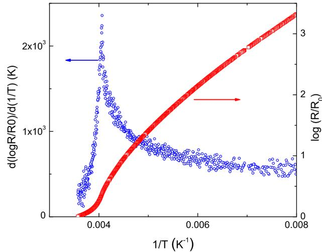
FIG. 1. Logarithm of the electrical resistance,  $R$ , normalized to the  $R_0 = R(300 \text{ K})$  (right axis, red) and its logarithmic derivative (left axis, blue) as a function of the inverse temperature.
