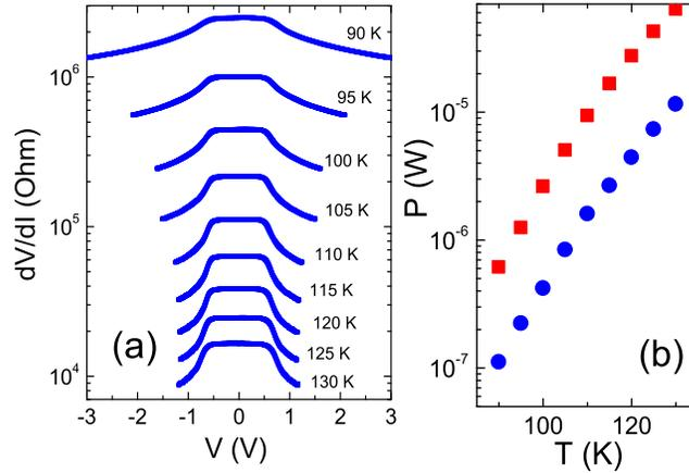
FIG. 2. (a) Differential current-voltage characteristics,  $dV/dI(V)$ , in one of the samples demonstrating the CDW collective motion in the temperature range 90-130 K; (b) Joule power dissipated at the threshold electric field,  $P(E_t)$ , (blue circles) and at twice the threshold,  $P(2E_t)$ , (red squares) as a function of temperature.
