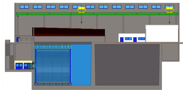
Figure 9: The ESS $\nu$ SB near detector layout. In the left picture, an artistic view of the detector is shown with an event happened in the sFGD. The trajectory of a positive muon (red) in the sFGD (bended by the magnetic field) and the two neutrinos (blue) from its decay in the WatCh are shown. Emitted Cherenkov photons in the WatCh are shown in orange. The right picture, presents an engineering design of the detector and the cavern.
