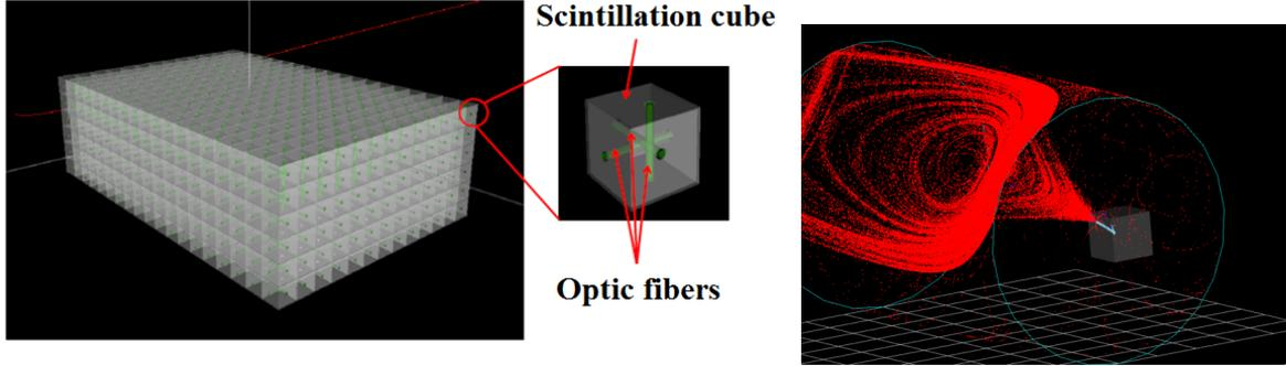
Figure 10: (Left) design of the Super Fine-Grained Detector with three-dimensional read-out. (Right) An  $\nu_\mu$  interaction event in the sFGD cube with a secondary muon producing a Cherenkov light in the near water Cherenkov detector.
