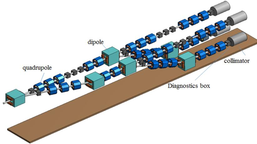
Figure 5: A 3D isometric view of the beam switchyard.
