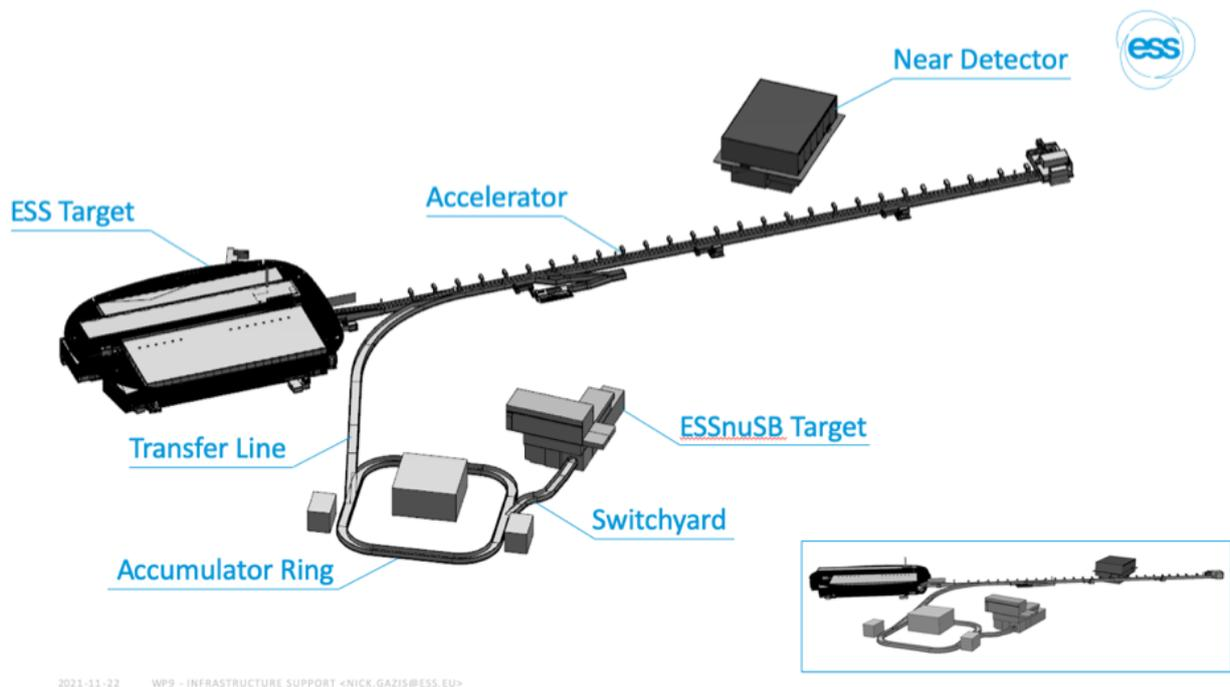
Figure 17: ESS building layout including the ESS $\nu$ SB buildings.
