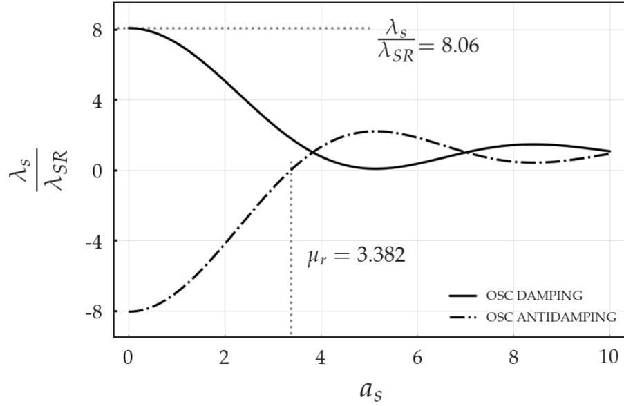
**Extended Data Fig. 3 | Computed dependence of damping rate on synchrotron amplitude for the measured OSC performance:** Total longitudinal damping (solid) and antidamping (dashed) rates as a function of normalized synchrotron amplitude. The rates are normalized to the strength of the longitudinal synchrotron radiation damping.
