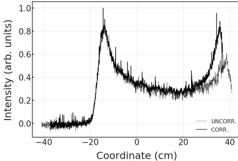
**Extended Data Fig. 2 | Correction of nonlinearity in streak camera image:** Longitudinal distribution before (dotted) and after (solid) correction of the streak-camera non-linearity for the OSC in the antidamping mode.
