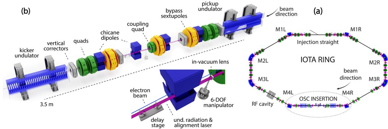
**Fig. 2|Schematic of the IOTA OSC system. a,** Schematic of the IOTA ring and the location of the OSC insertion. **b,** Diagram of the OSC insertion including the undulators, chicane and light optics (inset).
