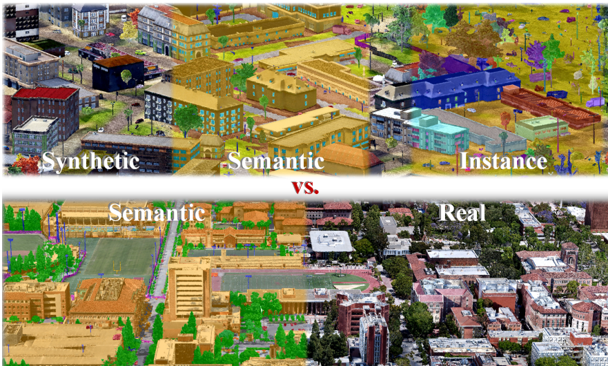
Figure 1: Example point clouds in STPLS3D dataset. Top row: synthetic point clouds with point-wise semantic and instance annotations. Bottom row: real point clouds captured from USC.
