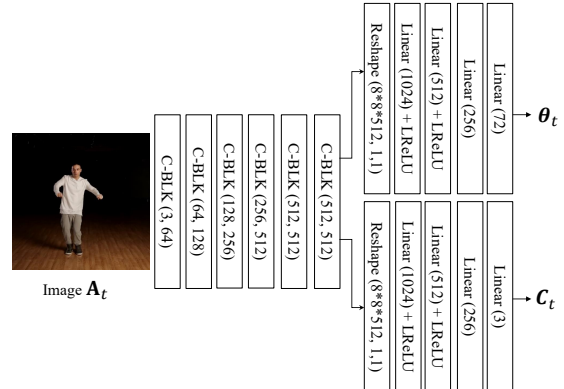
Figure 10. Network design for our 3D body and camera pose regression network ( f_{\text{track}} ). The details for C-BLK, D-BLK, Conv, and LReLU are described in Figure 11.
