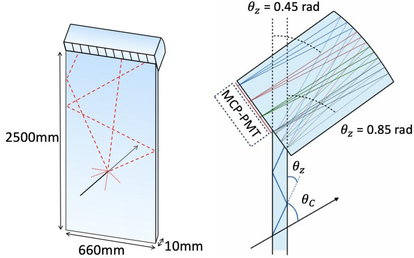
Figure 1: Sketch illustrating a single TORCH module. Charged hadrons traversing the quartz plate emit Cherenkov photons, which are propagated to the edge of the detector via total internal reflection. The photons are focused by a cylindrical mirror onto a detector plane comprising 11 MCP-PMTs, when fully equipped. The position of a photon along the MCP-PMT is used to infer the photon Cherenkov angle.
