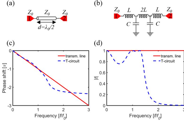
Figure S5. Phase and amplitude of the transmission coefficient comparison between the (a) transmission line and (b) double T-circuit.
