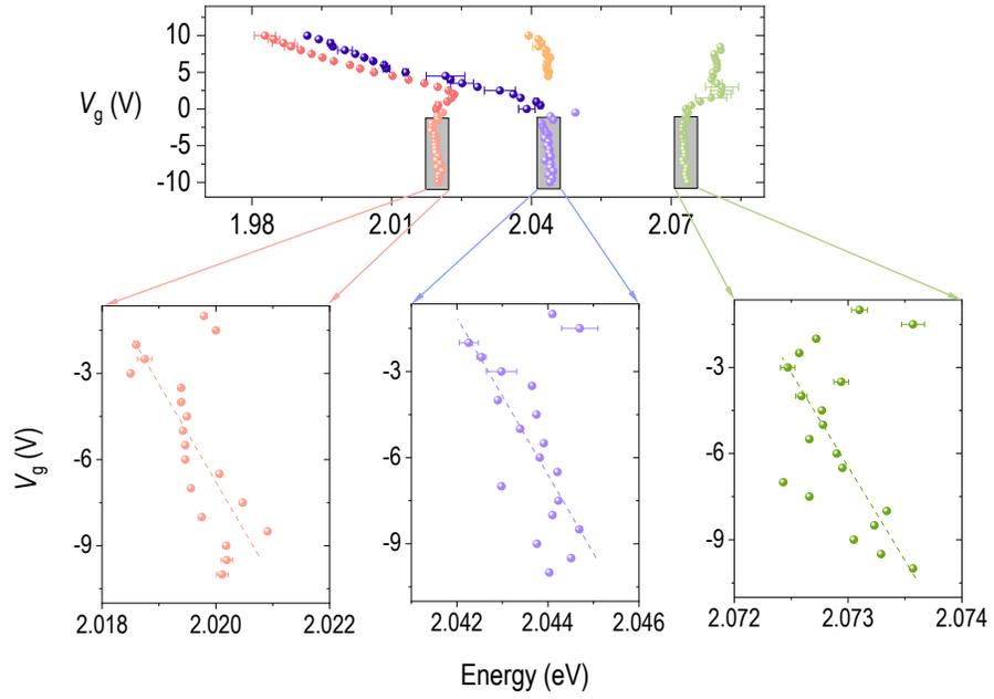
FIG. 3. **Blue shift of exciton, positive trion and positively charged biexciton.** We note about 2-4 meV blue shift of  $\chi^0$ ,  $\chi^+$  and  $\beta^+$  (from left to right). The dashed lines are guide to the eye.
