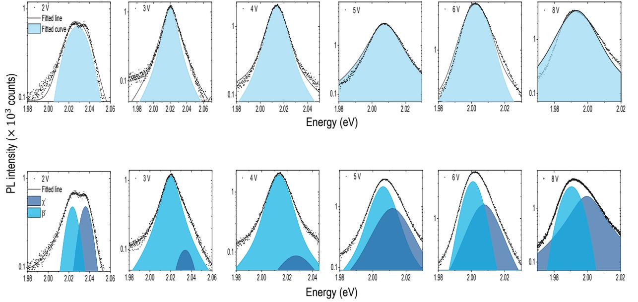
FIG. 6. **PL fitting comparison for the trion and charged biexciton merged peak with a single and double voigt curve.** We fit the  $\chi^-$  and  $\beta^-$  merged PL peak (in the  $2 \leq V_g \leq 8$  V range) with a single as well as two voigt curves. Fitting with two voigt curves improve the fit quality significantly, proving existence of both  $\chi^-$  and  $\beta^-$  even after strong spectral overlap.
