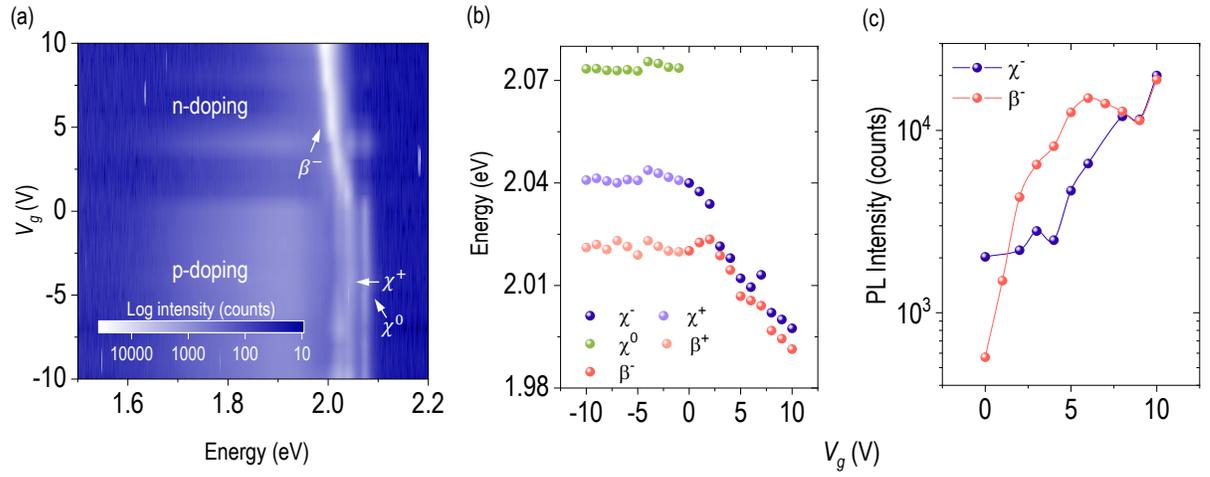
FIG. 8. **Continuous wave PL fitted peak position and intensity.** (a) PL data obtained using a 532 nm continuous wave laser is shown in a color plot. (b) Fitted peak positions showing spectral overlap between  $\chi^-$  and  $\beta^-$ . (c) Fitted peak intensity values showing no appreciable reduction of  $\chi^-$  PL intensity, even in the spectral overlap region.
