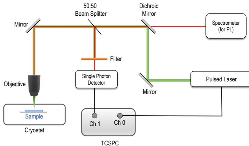
FIG. 1. **Schematic of the measurement setup for *in situ* TRPL and steady-state PL.** A pulsed laser source (pulse width  $\sim 48$  ps) of 531 nm wavelength and 10 MHz repetition rate is used for excitation. A temperature of 5 K is maintained in the cryostat during measurement.
