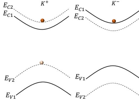
FIG. 5. **Schematic of intervalley trion configuration.** We observe an intervalley trion after  $V_g > 4.5$  V, schematically depicted here. The extra electron along with the spin allowed bright electron-hole pair is taken from the top conduction band of the other valley.
