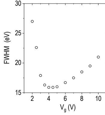
FIG. 7. **FWHM of the merged PL peak versus gate voltage.** The FWHM of the merged PL peak of  $\chi^-$  and  $\beta^-$  together is plotted with  $V_g$ . It shows a non-monotonic behavior with the minimum FWHM obtained when the overlap between trion and charged biexciton is maximum.
