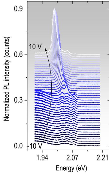
FIG. 2. **PL spectra at different gate voltages.** The PL spectra obtained at  $V_g = -10$  to 10 V. In the p-doping regime ( $V_g < 0$  V) three PL peaks namely  $\beta^+$ ,  $\chi^0$  and  $\chi^+$  (refer to main text Figure 1) do not show any sharp spectral shift, whereas in the n-doping regime ( $V_g > 0$  V),  $\chi^-$  and  $\beta^-$  show strong redshift including a spectral overlap region.
