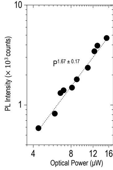
FIG. 4. **Power law fitting of charged biexciton with respect to laser power.** We fit the obtained charged biexciton PL intensity (at  $V_g = 0$  V) with varying incident laser power. Fitting shows a super-linear relation of PL intensity of  $\beta^-$  with laser power ( $\propto P^{1.67 \pm 0.17}$ ).
