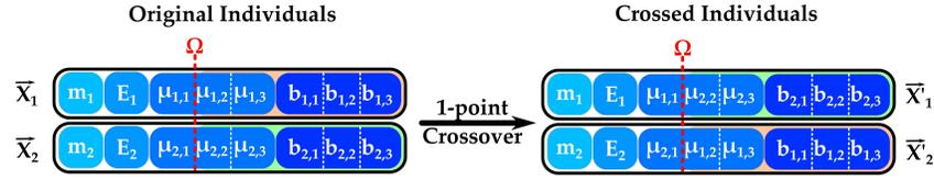
Fig. 6: Single-point crossover applied on FL-COP solutions
