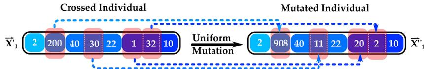
Fig. 7: Uniform mutation applied on FL-COP solutions
