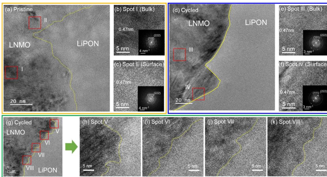
**Figure 4. Interfacial nanostructure and morphology at the LNMO/LiPON interface**(a) Cryo-TEM image of pristine LNMO/LiPON interface and (b) zoomed LNMO images of bulk (inset; FFT image) and (c) surface (inset; FFT image). (d) Cryo-TEM image of cycled LNMO/LiPON interface and (e) zoomed LNMO images of bulk (inset; FFT image) and (f) surface (inset; FFT image). (g) Another cryo-TEM image of cycled LNMO/LiPON interface and (h-k) zoomed interface images at different spots.
