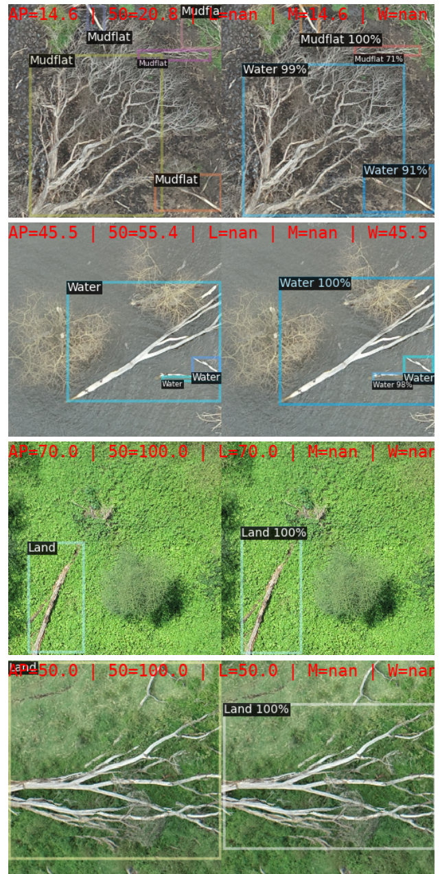
Figure 5. Sample results from different scenes using Faster-RCNN, with average precision (AP) averaging over all IoU levels in [0.5, 0.95], step size 0.05 and (50 being precision at \text{IoU} \geq 0.5 ) on three classes: Dead Tree in Water (W), on Land (L), and on Mudflat (M). Ground truths are shown on the left and predicted bounding boxes on the right. The confidence levels (%) are shown on the bounding boxes.
