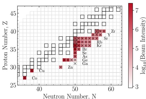
**Figure 8.** Target nuclei which  $(\alpha, n)$  reactions affect elemental abundance ratios in different astrophysical conditions indicated with an x-mark. The color-code corresponds to estimated intensities of reaccelerated beams at the second FRIB PAC (Tarasov 2020).
