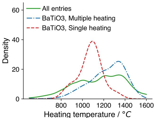
Figure 8: The curves are the distribution of heating temperatures for each group of reactions in the training dataset. The dashed/dotted lines show temperature distributions for the reaction  $\text{TiO}_2 + \text{BaCO}_3 \rightarrow \text{BaTiO}_3 + \text{CO}_2$  (red dashed line for single-heating reactions and blue dotted line for multiple-heating reactions). Green solid line shows the temperature distribution for the entire dataset.
