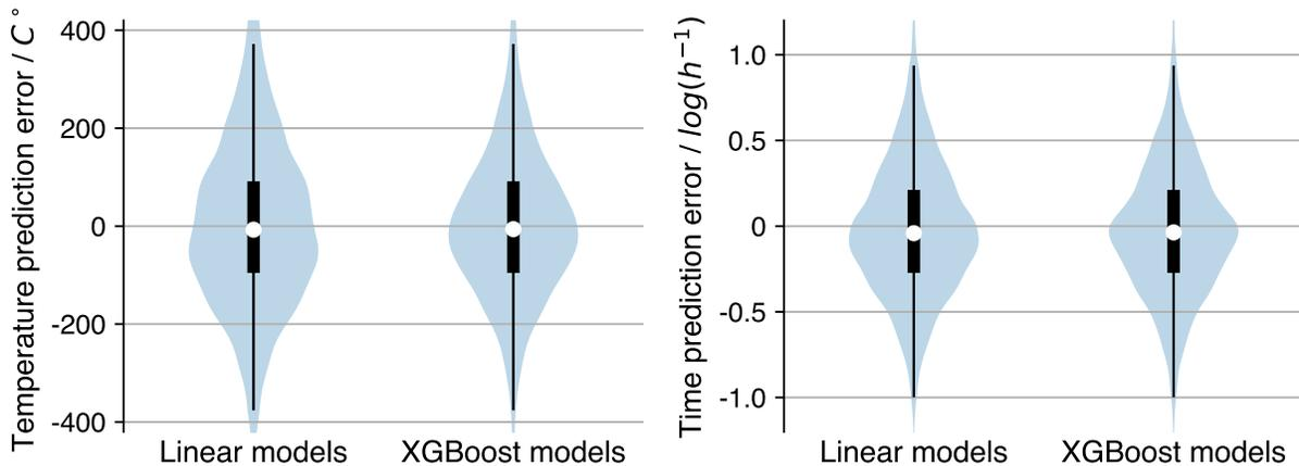
Figure 6: LOOCV prediction error distributions of synthesis temperature and time. Plotted are prediction median values (shown with white dots), interquartile ranges (IQR, or the spread of errors between 25% and 75% percentiles, shown with thick lines), and 1.5x IQR (shown with thin lines). Shaded areas are probabilistic density estimations of the errors. Our models are expected to make prediction errors within the IQR half of the times and within the 1.5x IQR most of the times.
