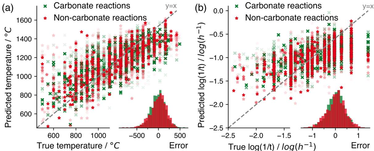
Figure 3: Regression result of linear models. The scatter plots show reported conditions v.s. predicted conditions for temperature prediction (a) and time prediction (b). Opacity of the markers indicates the weights of data points. Histograms of prediction errors are also shown.
