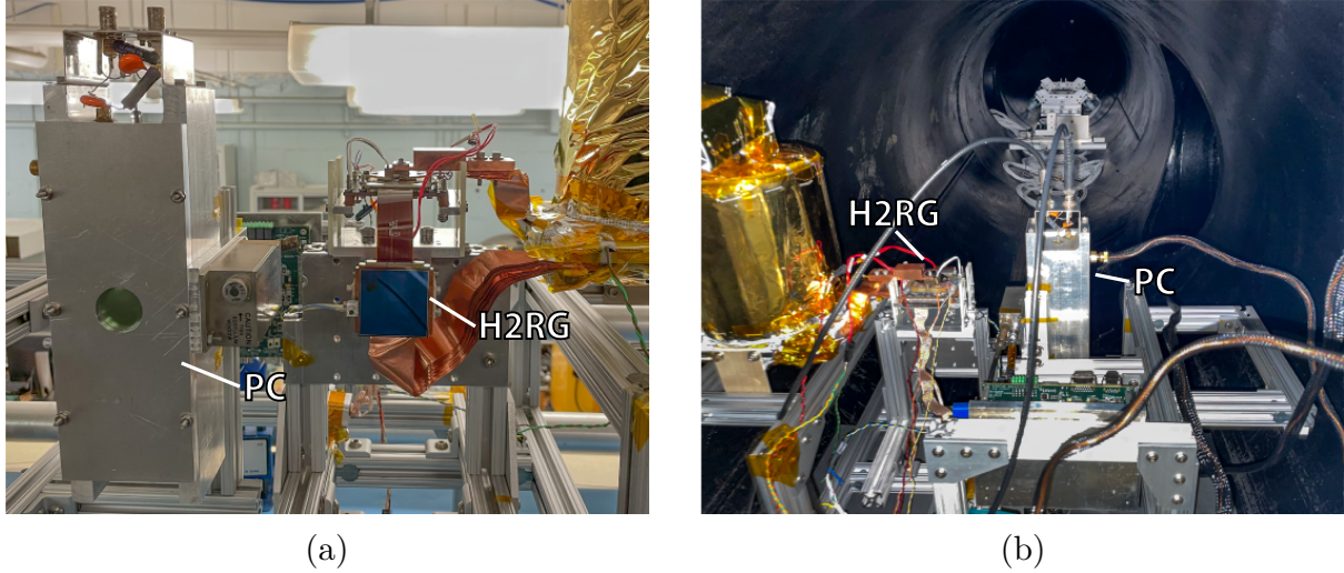
Fig 3 The front of the detector mounting structure shown outside the vacuum chamber (a), with the PC (left) and the H2RG (right), and the back of the same structure shown in place for the QE measurements inside the beamline (b). A Si PIN diode detector was also mounted between these detectors but was not used during QE measurements.
