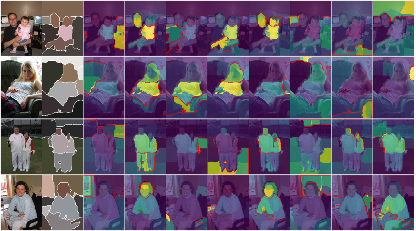
Figure 8. The multi-head attention maps reveal the fine-to-coarse semantic relationships among image segments. From left to right: input image, our feature-induced segmentation, attention maps in the decoder of our clustering transformers. We use a clustering transformer to partition each image into 8 clusters, and show the attention map (colored in viridis color maps) of each cluster to all the image segments. We observe these clusters correlate better with image segments that carry more similar semantic meanings, e.g., the ‘head’ cluster attends more to body parts than background regions. Such correlation information implies the next-level groupings: ‘head’ will be grouped with ‘torso’ instead of ‘background’
