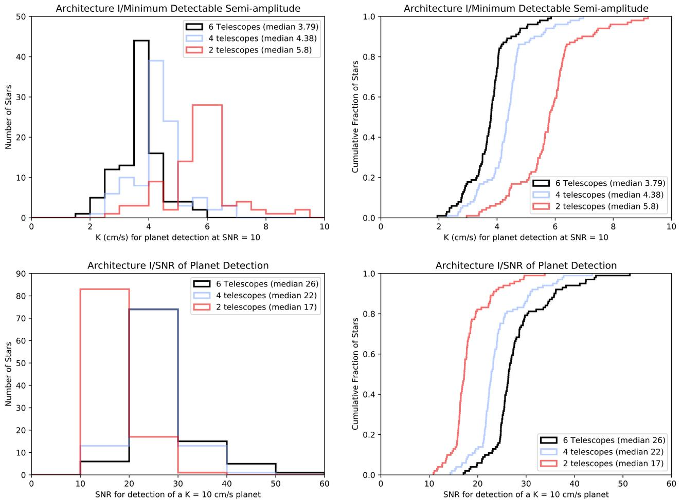
**Figure 11.** Histograms of our sensitivity calculations from the observations. Top: smallest semi-amplitude  $K$  for which a planet with a period much shorter than our 10 year survey could be found at an SNR of 10. Bottom: The SNR at which a planet with a period much shorter than our 10 year survey could be detected at if it had a semi-amplitude of 10 cm/s. In both cases, these values are calculated from equation 1.
