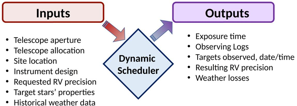
**Figure 1.** Outline of the simulation pipeline, including the exposure time calculator (ETC) and dispatch scheduler.
