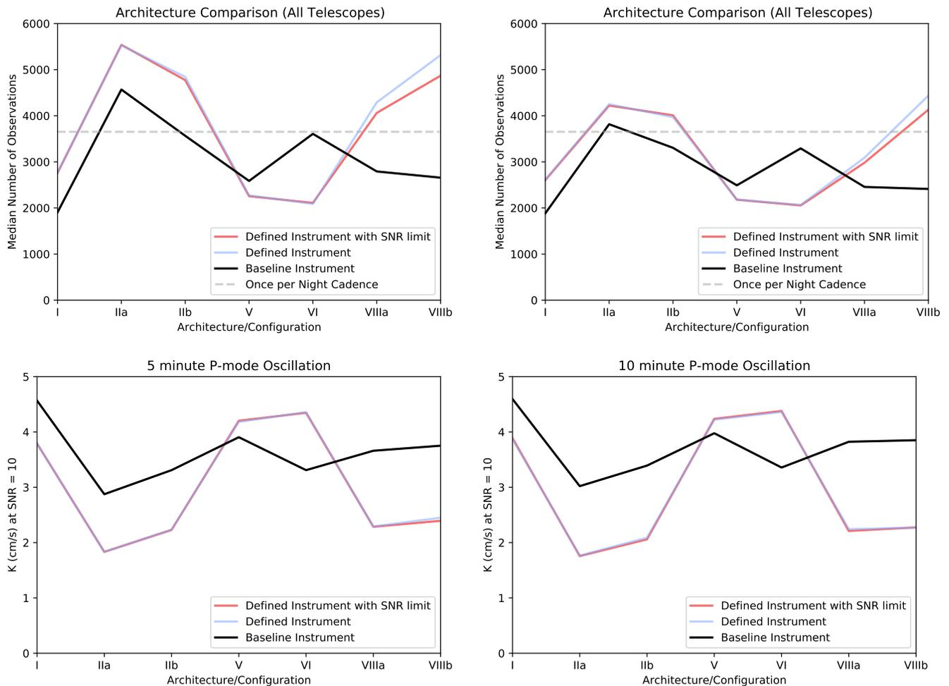
**Figure 16.** Comparison across architecture simulations and P-mode oscillation assumptions for median number of observations (top), and minimum reflex velocity semi-amplitude sensitivity (bottom). The 5 minute (left) and 10 minute (right) graphs use the same vertical scale for ease of comparison.
