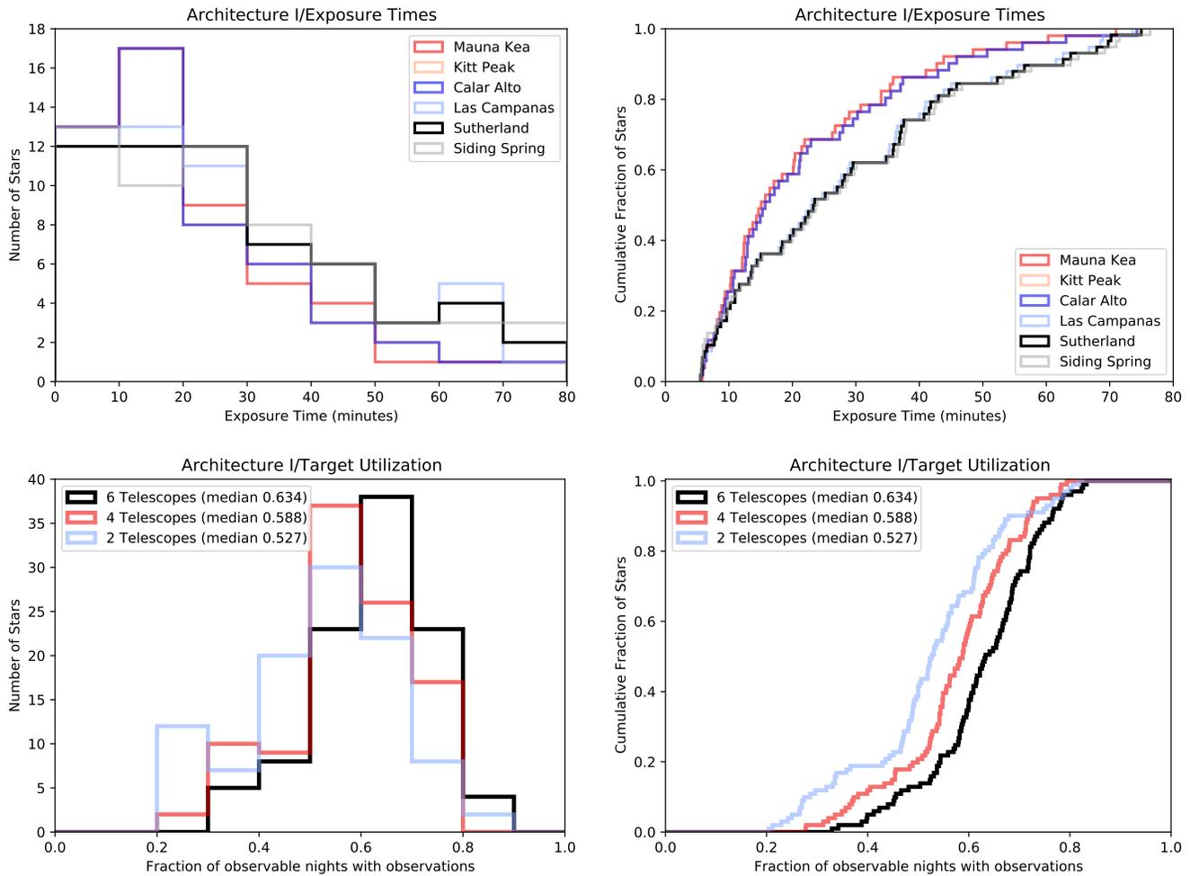
**Figure 10.** Top: Histograms of exposure times per star calculated individually at each site. Bottom: how “efficiently” each star was observed. That is, for what fraction of nights where a star could be observed from at least one site it was observed at least once.
