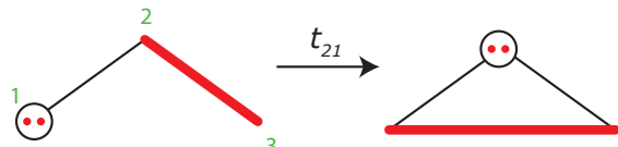
FIG. S14. Effect of the electron hopping operator, moving an electron from atom 1 to atom 2. The amplitude of such a hop is the Hückel parameter here denoted t_{21} . Note, that the singlet bond originally at atoms 2 and 3 moves to atoms 1 and 3.
