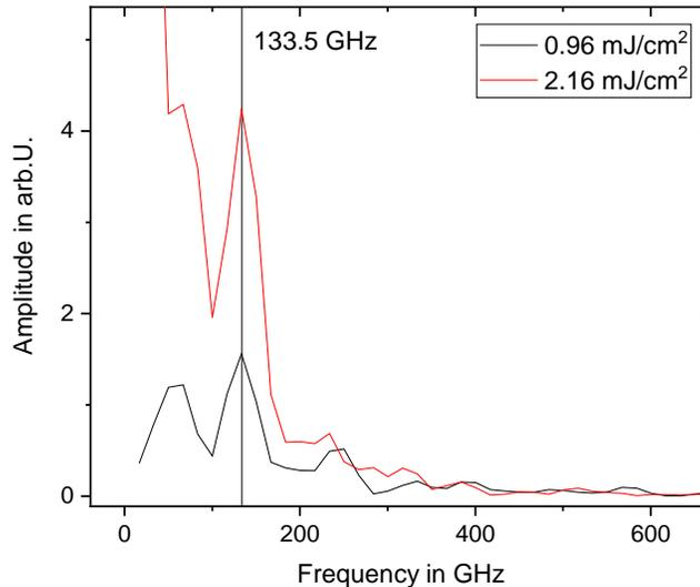
FIG. S3: Power spectrum of the time-resolved MOBF traces obtained for high fluences. The marked frequency of 133.5 GHz indicates the appearance of the low-frequency magnon mode in NiO.
