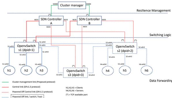
FIGURE 10. RECS - a SDN-Based system under evaluation. This system aims to beneficially manage the runtime adaptation of computational resources from edge cloud systems to mitigate against disruptive events on these systems
