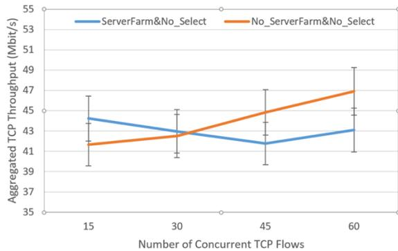
FIGURE 14. Performance comparison between the single server scenario and the server farm instance
