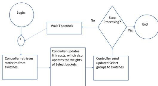
**FIGURE 9.** Control loop that retrieves statistical information from switches, enables the controller to update link costs and the weights of Select buckets, which follow the parallel cost paths to each specific destination, and then ends with the controller sending renewed Select groups to the switches. These groups allow load balancing at the data forwarding level. The loop reruns periodically (once every T seconds)
