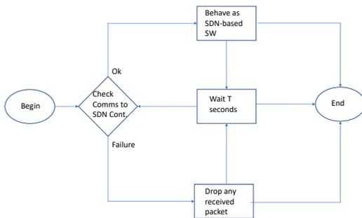
**FIGURE 3.a** OpenvSwitch secure operation mode after the switch becomes disconnected from the upper SDN controller
