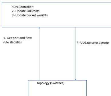
**FIGURE 6.** Design of solution to mitigate link congestion based on the collection of switch statistics by the SDN controller, update of link costs and bucket weights, and transfer of renewed select groups from the SDN controller to the controlled switches
