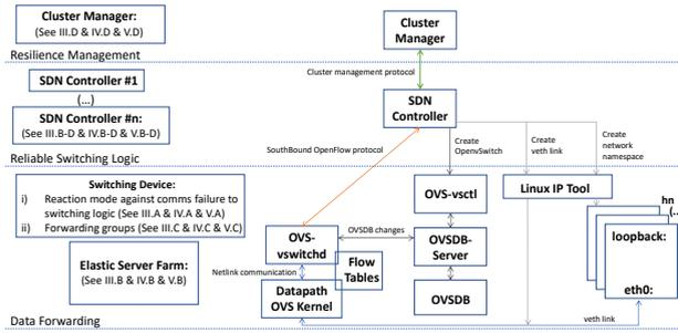
**FIGURE 2.** Architectural layout of the proposed cross-level programmable solution (RECS) to enhance the system’s operational resilience against both communications failures and congestion in edge computing domains. Inside each block at the left are the paper sub-sections that discuss the key block functionalities and their evaluation
