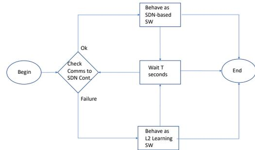
**FIGURE 3.b** OpenvSwitch standalone operation mode after the switch becomes disconnected from the upper SDN controller
