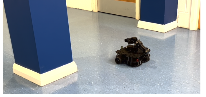
Fig. 5: TurtleBot3 Waffle Pi Robot and the Office Environment
