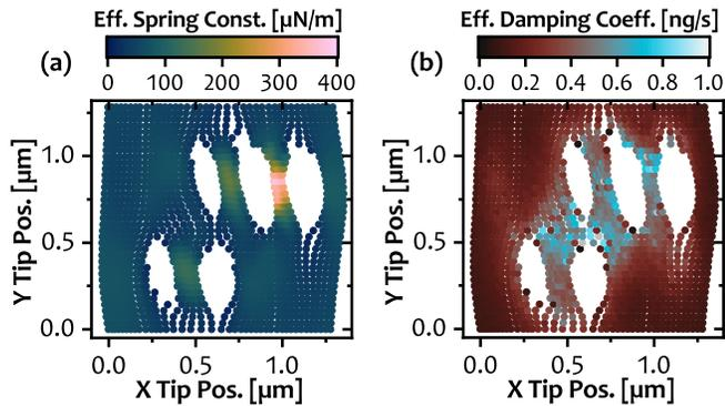
FIG. 6: Dependency of (a) effective spring constant and (b) effective damping coefficient on  $x$  and  $y$  position at  $\Delta z = 30$  nm. The data was obtained simultaneously with the MRFM signal shown in Fig. 3.
