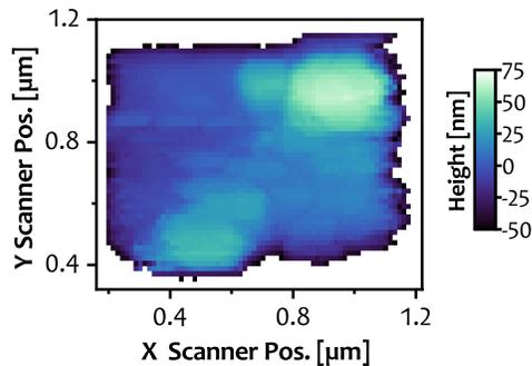
FIG. 9: Topography scan of the 870 nm x 630 nm rectangular cantilever apex with the attached virus samples. The scan was performed at room-temperature after performing the 3D MRFM scan.
